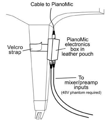
Figure 16. Attaching the Pouch to the Piano Leg.
