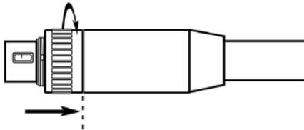
3. Next, rotate the collar two turns in the opposite direction (moving it away from the connector cover toward the connector pins). (Fig. 1-C)
