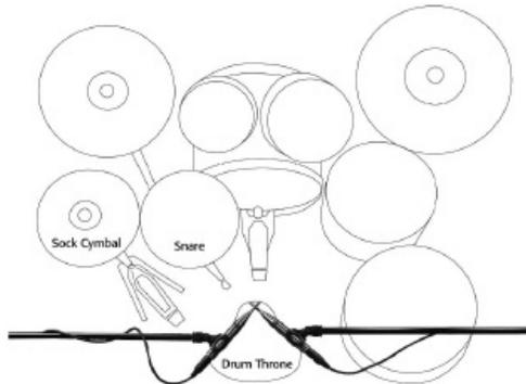
Figure 1. Overhead miking with HORIZONTAL X/Y positioning
