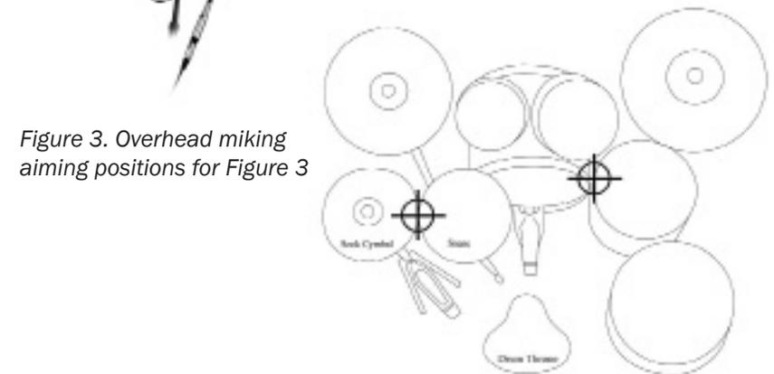
Figure 3. Overhead miking aiming positions for Figure 3
